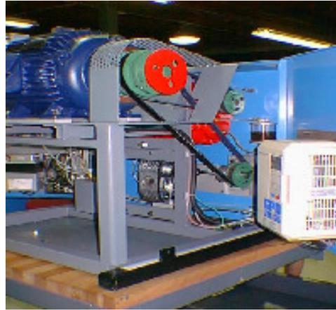
**The unit is equipped with two blowers, low range and high range. During high range, both blowers are activated. The clutch is manually operated.**
